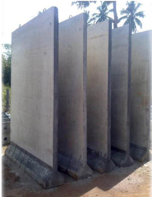
Fig. 1. Precast RCC Wall Panels
